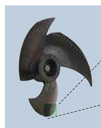
Escaping eddies are sucked in by the bent blade edges, reducing overall turbulence.
